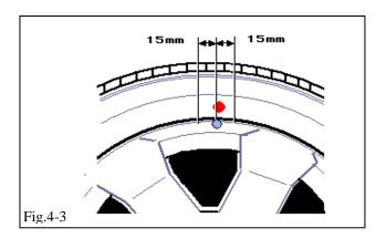
(f) Remount the OE tire on the alloy wheel, matching tire high spot (red dot) with that of wheel low spot (blue sticker). Ensure the marked side is facing inward.
